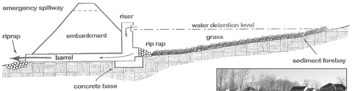
Dry ponds are the most common stormwater management facilities in Northern Virginia. Most do not contain a permanent pool of water and no water should remain if it is functioning properly.
