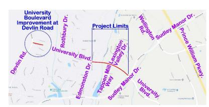
**PURPOSE:** To provide a connection of University Boulevard and construct a two-lane roadway with median curb, curb and gutter, and sidewalk.
